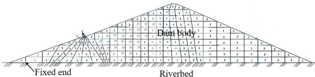
Figure 3. Schematic diagram of a dam structure analysis model, where the riverbed is assumed to be continuous, rigid, and steady-state.
