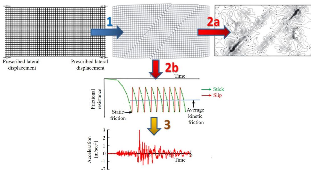
Figure 1. Tectonic plate-induced shear band formation process and ground vibration under lateral compression (Hsu, 2018).
